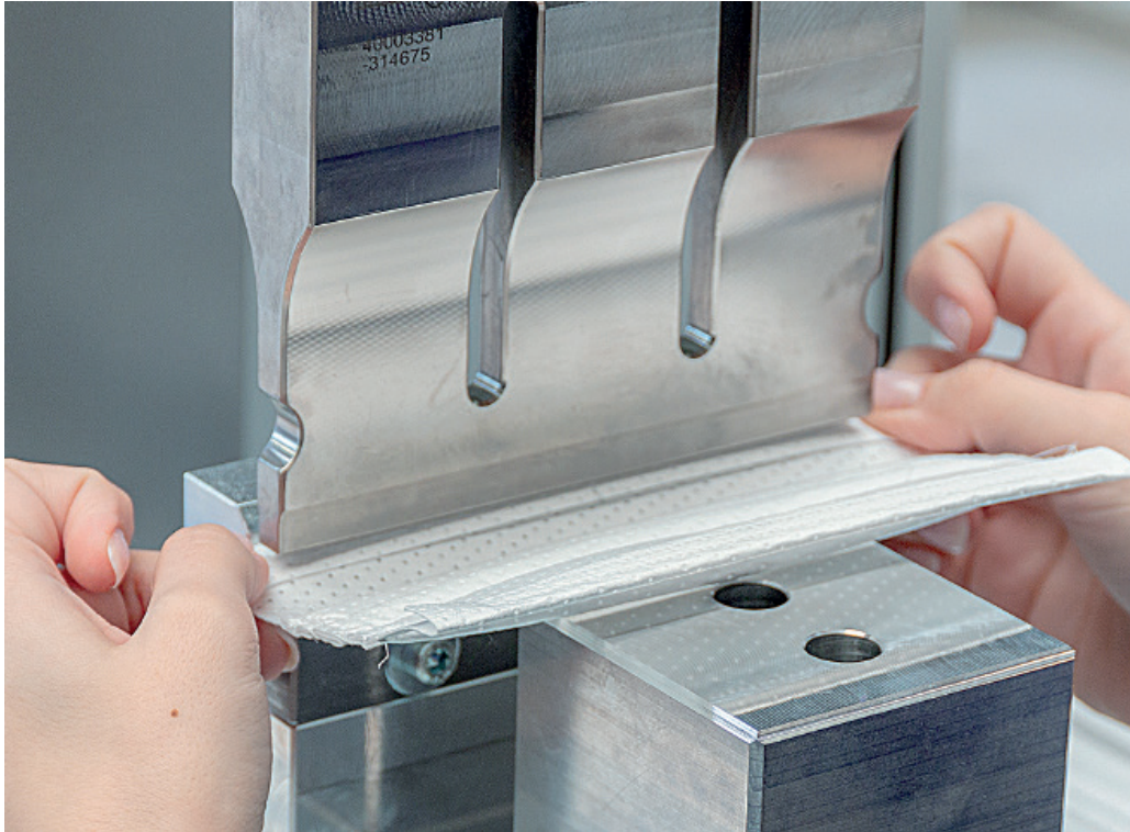
3. Horizontal ultrasonic welding of cross seams 1 and 2. The nose band is slid in manually (no illustration). © Copyright SONOTRONIC Nagel GmbH
